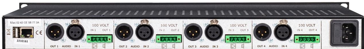
The Station Audio Control (SAC) is specifically developed for monitoring and surveillance of PA speaker networks, for example on railway station facilities. It enables measuring of audio levels from both the line inputs and amplifier outputs of (100 Volt) amplifiers. Deviations from preset values are signaled and reported, e.g. to a server via an SNMP trap.
